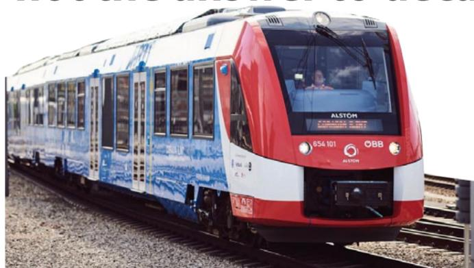
**ALSTOM CHALLENGER:** This is the Coradia iLint train, in regular service near Vienna in Austria last year. The iLint is built by Alstom in Germany and can be diesel-powered. It also uses on-board fuel cells to convert hydrogen and oxygen into electricity, reducing operating emissions to zero.
