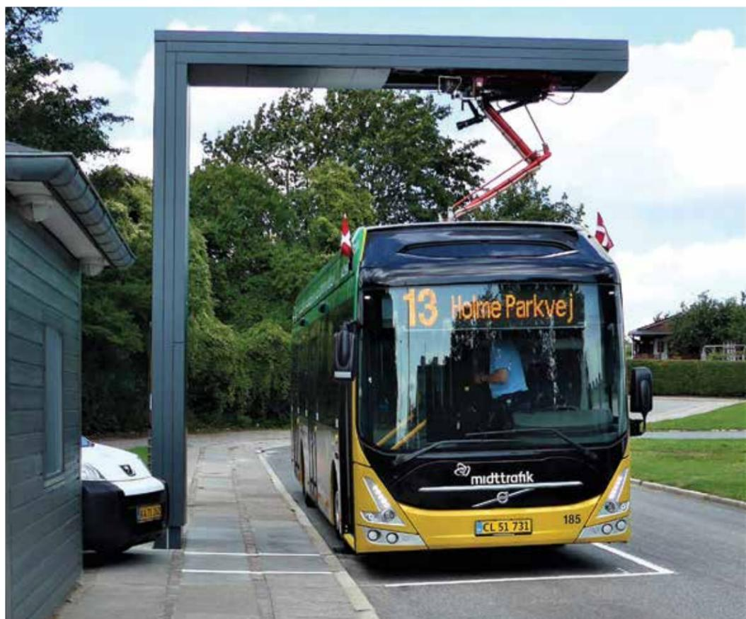
**ELECTRIC CHARGE:** A quick charge keeps Aarhus' new bus going until it can get back to base
