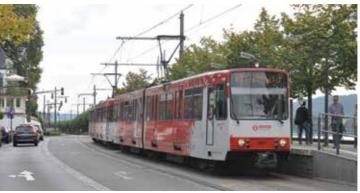
THE FLEXIBILITY OF LIGHT RAIL: Route 66 in Bonn travels underground in the city centre, but surfaces on segregated tracks in the suburbs, and as seen here in Konigswinter, on a single track, sharing space with road traffic
