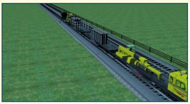
Module 1: Piling and structures installation. Module 1 would consist of four parts, two master vehicles both capable of operating as either a piling vehicle or a structures mounting vehicle and two flatbed match wagons for transporting at least 15 piles and at least 15 mast structures. The module can be split, providing two separate piling-structures vehicles.
