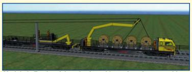
Module 2: Feed-aerial earth wire cable, registration assembly. This module comprises three vehicles. One master vehicle will house eight cable drum carriers and two manipulator arms capable of positioning the cables behind, above or in front of the masts. One slave vehicle will be fitted with welfare facilities and a mobile elevated working platform basket for attaching the cables to the mast. The second master vehicle is fitted with racking, a crane and an elevated working platform basket.
