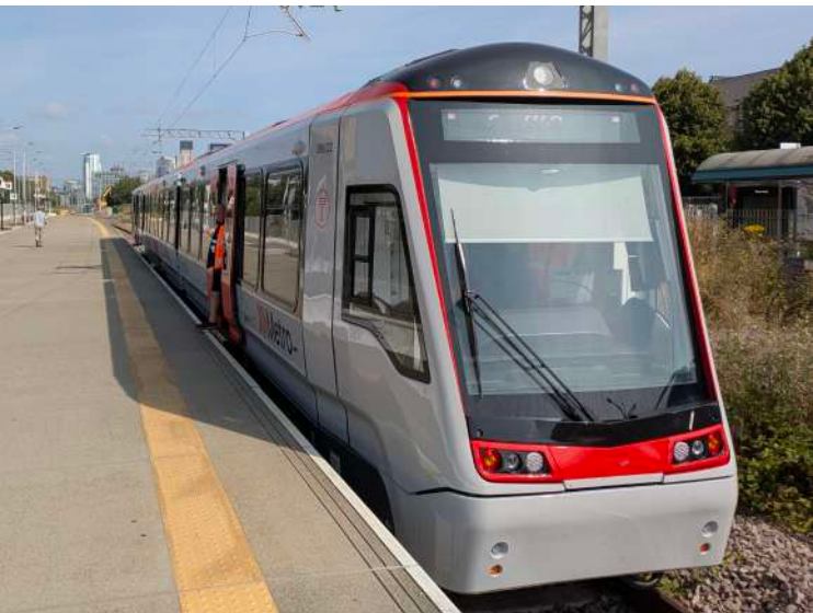
A new class 398 tram-train at Cardiff Bay station in August. These units are powered by overhead line or battery. The station is currently being expanded to include a second platform and track to the left. This part of the line is to be converted to line-of-sight tram operation
