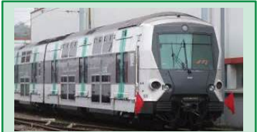
EXAMPLE: The latest Paris RER train is double-deck but with three entrance doors per car
