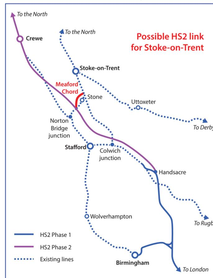
**HS2 OPTION: Stoke-on-Trent is keen to share the benefits of high speed rail and believes a five-mile Meaford chord could deliver a double-barrelled economic impact from HS2 – for both Stoke and Crewe. It is working with the Department for Transport on the idea which has a 'better benefit to cost ratio than any other current UK rail project'**
