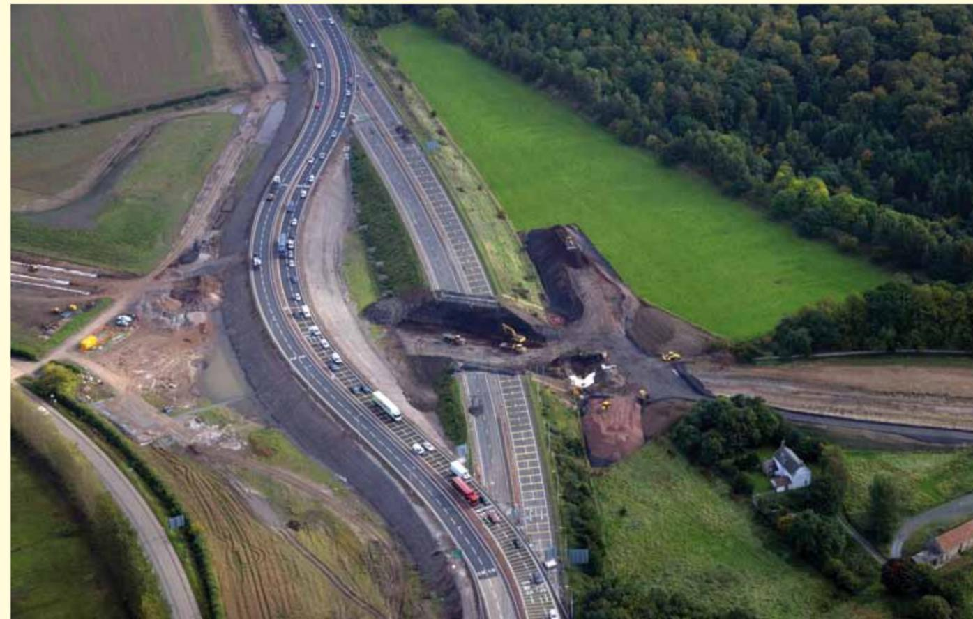
**Rail investment in Scotland is high. The busy Edinburgh southern by-pass road is temporarily diverted at Sherriffhall to allow a bridge to be constructed as part of the programme to reinstate the Borders Railway. Once the bridge is complete, the road will be moved back to its original alignment**
