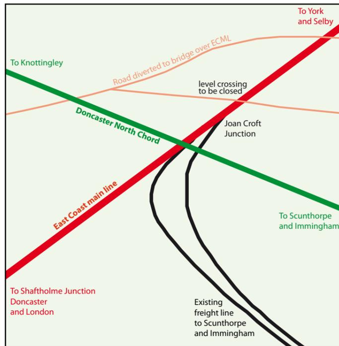
**DIAGRAM OF PAGE ONE PICTURE:** The new chord allows freight to travel across the East Coast main line without impeding main line traffic while the newly diverted road allows the level crossing near Joan Croft Junction to be closed
