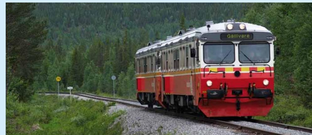
**RUGGED:** One of the Inlansbanan's diesel-hydraulic railcars made by Fiat/Kalmar
