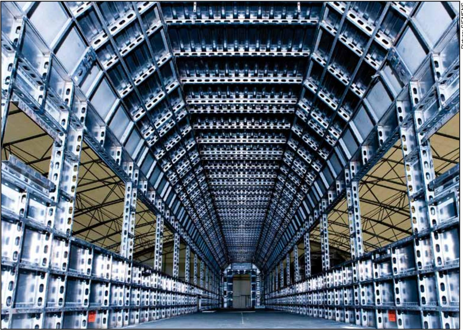
**SKELETON:** The bodyshell of Austrian Federal Railways' Railjet vehicle, made of steel which makes it easy to recycle
