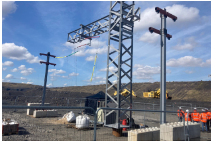
The composite twin track cantilever (CTTC) in two-track configuration, set up for weight testing at the Global Centre for Rail Excellence
