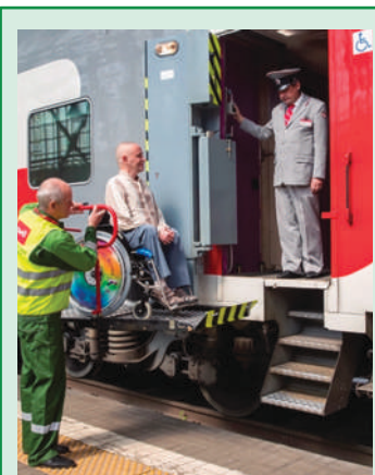
BIG STEP: A wheelchair lift as used on Russian Railways
