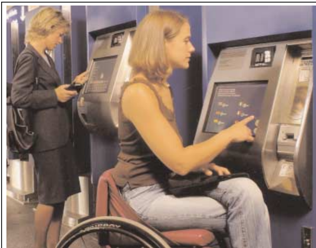
A new generation of customer-friendly ticket machines are under test at stations in England. They are designed to be used by disabled people but should make buying a ticket easier for everyone. Designers had to give special thought to the angle of the touch screens, the position of money and credit card slots as well as ticket and change dispensers. The machines, made by Ascom - with input from designers Hothouse Product Development Partners - are at Gatwick Airport, Marylebone, Haslemere, Wokingham, East Croydon, Haywards Heath, King's Cross, Elstree and Loughborough.
