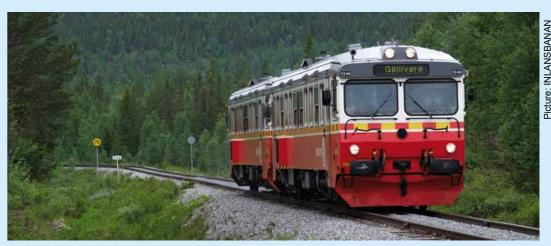
RUGGED: One of the Inlansbanan's diesel-hydraulic railcars made by Fiat/Kalmar
