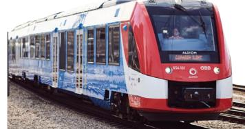
ALSTOM CHALLENGER: This is the Coradia iLint train, in regular service near Vienna in Austria last year. The iLint is built by Alstom in Germany and can be diesel-powered. It also uses on-board fuel cells to convert hydrogen and oxygen into electricity, reducing operating emissions to zero.
