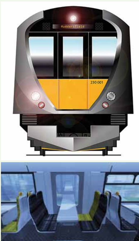
Vivarail's new-for-old D-Train, above. Lower picture: A seating and glazing unit which replaces the sliding door entrance on the original trains
