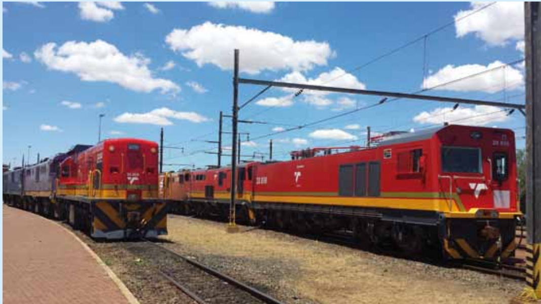
HEAVY METAL: Two new class 20E electric locos (right) at Kimberley, with, on the left, South Africa’s standard branch line class 35 diesel, built by America’s General Motors in the 1970s
